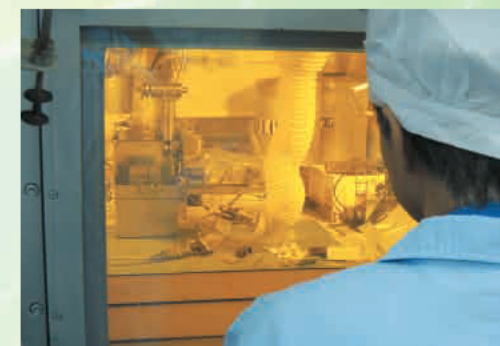
Remote handling of specimen in hot cell
