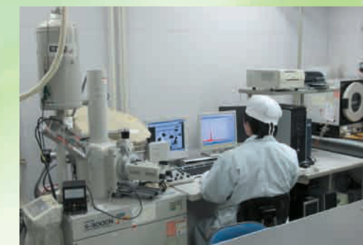
Analysis by scanning electron microscope(SEM)
